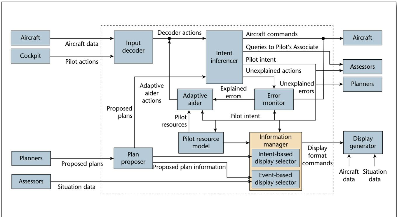
Figure 6. Flowchart of the Demo 3 Pilot-Vehicle Interface.
