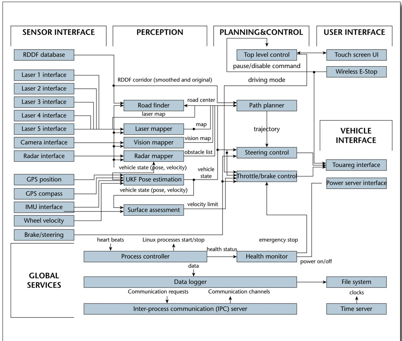
Figure 5. Flowchart of the Stanley Software System.
