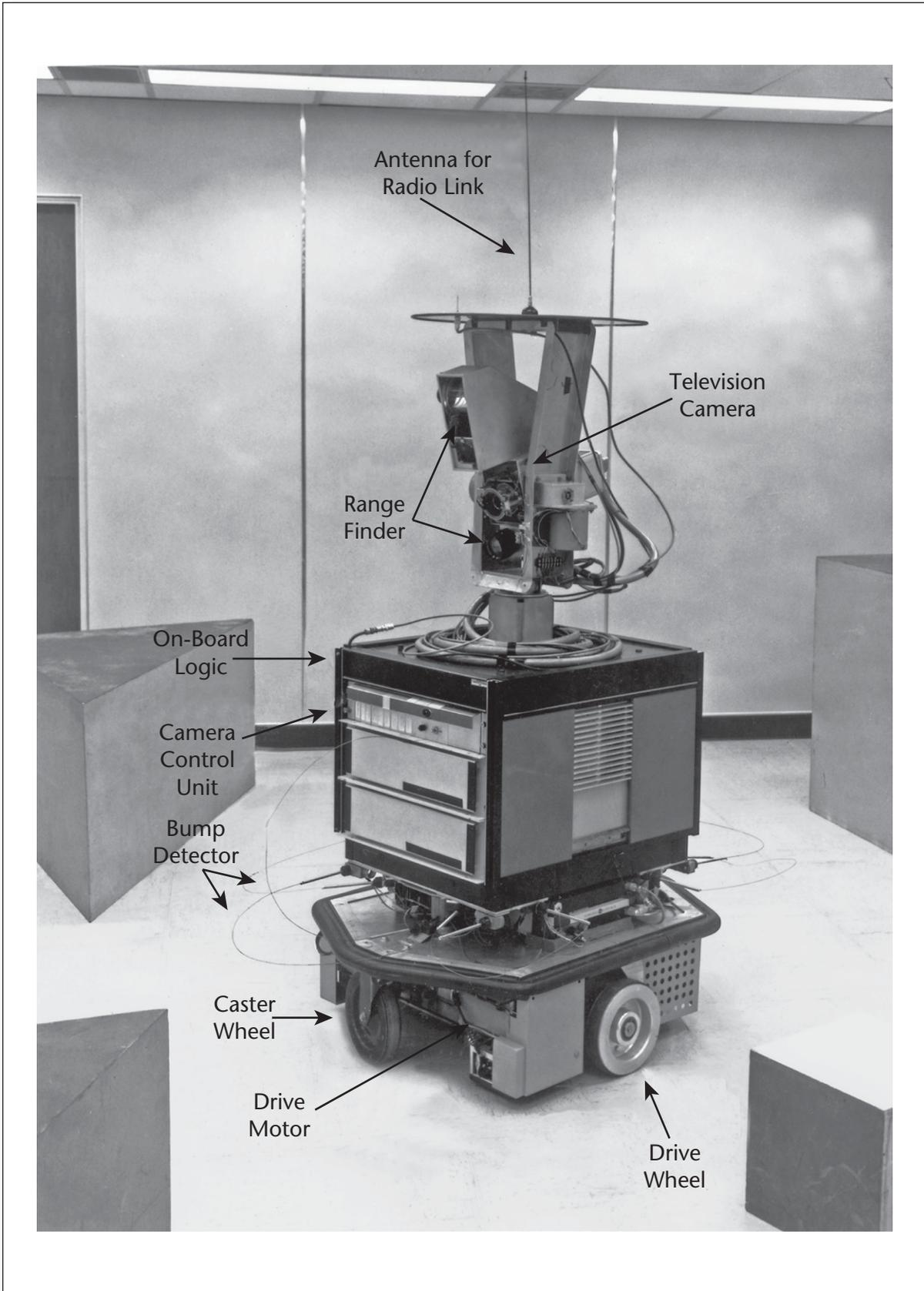
Figure 3. Shakey the Robot.
