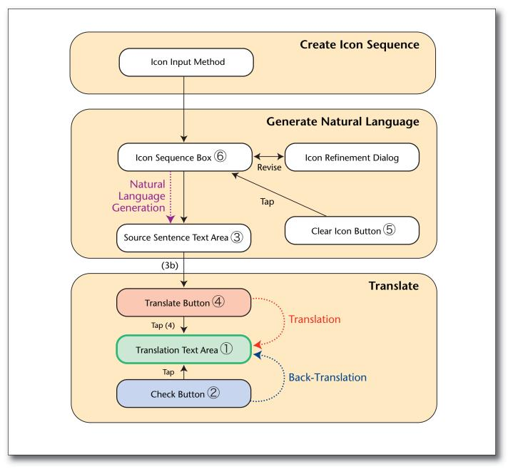
Figure 4. A Flow Diagram for the User Interface.
