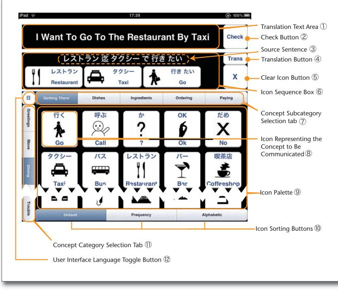
Figure 5. The Annotated User Interface for the picoTrans System.
