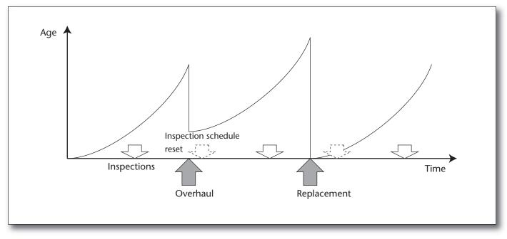
*Figure 3. Synchronized Replacements or Overhauls and Inspections, Resulting in the Elimination of Unnecessary Inspections (dotted).*
