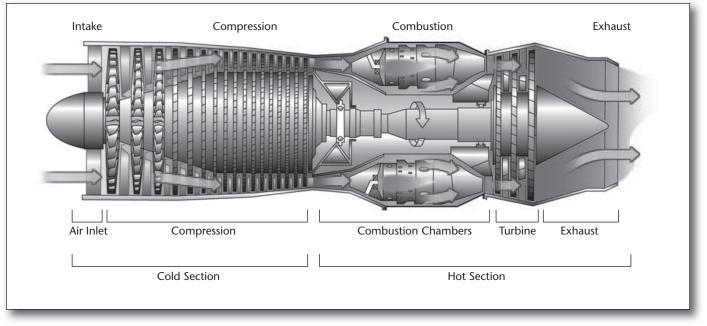
Figure 1. Schematics of a Gas Turbine.
