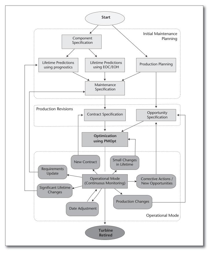
Figure 4. Workflow of Maintenance Planning using PMOpt.
