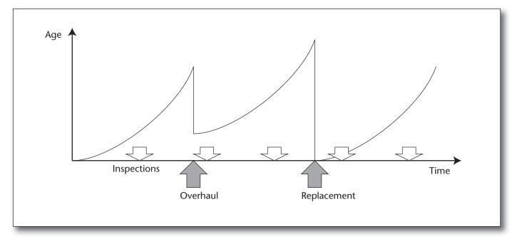
Figure 2. Unrelated Replacements or Overhauls and Inspections of a Single Component.
