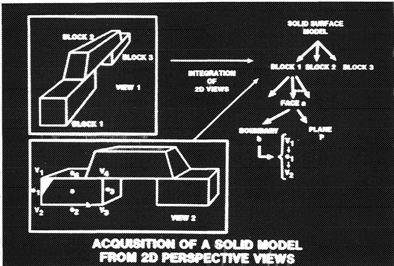
Acquisition of a solid model of a three-dimensional object from two-dimensional perspective views.
