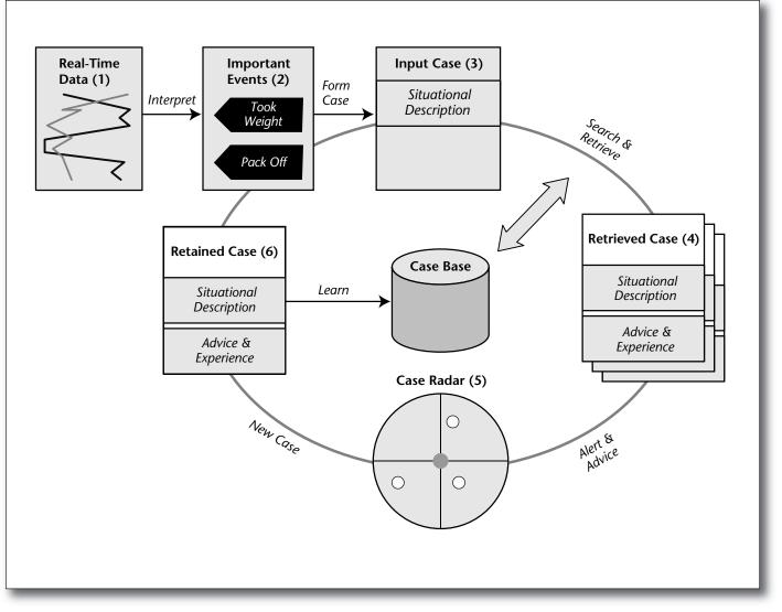
Figure 1. The DrillEdge CBR Cycle.
