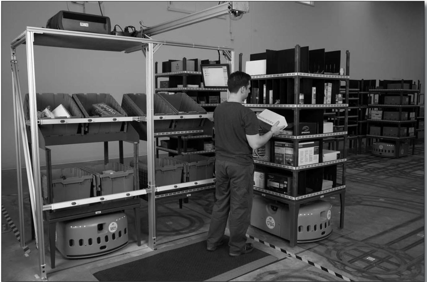
Figure 5. An OrderFetch Station in Which the Worker Fills Totes from Inventory Pods.
