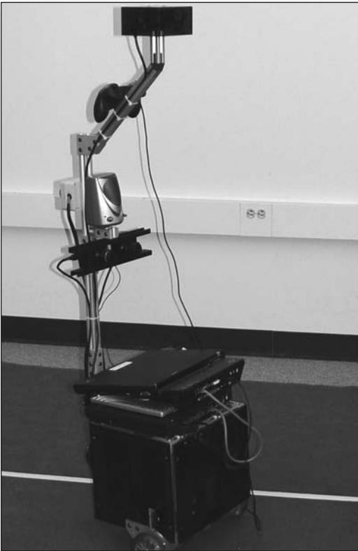
Figure 12. CMAssist, from Carnegie Mellon University, Demonstrated Person Detection, Tracking, and Interaction.
