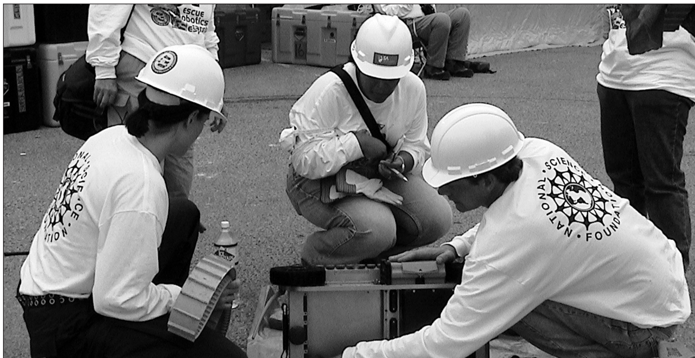
Figure 3. Scientists Participated in All Aspects of the Response, Including Decontaminating Robots from Dirt (and Possible Biological Residue from Ruptured Sewers or Body Fluids).
