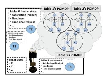
Figure 1: The robot operates in a restaurant with 3 tables, T1, T2, and T3. The robot builds a POMDP model for each table in the restaurant by using its own state and service actions, the table's state and the human's state. The robot has N POMDP models for a restaurant with N tables.
