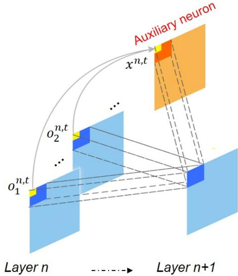
Figure 2: **Illustration of NeuNorm.** Blue squares represent the normal neuronal FMs, and orange squares represents the auxiliary neuronal FMs. The auxiliary neurons receive lateral inputs (solid lines), and fire signals (dotted lines) to control the strength of stimulus emitted to the next layer.
