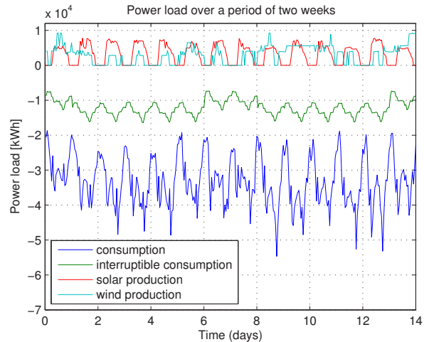
Figure 1: Two weeks of energy usage data for different customer types in a simulated environment.
