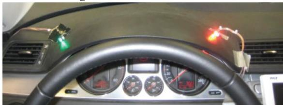
To further enhance the vehicle-driver interaction and to express more information to the user, an unsafe blinking algorithm is implemented. If it is unsafe to change lanes on a given side, the red LED not only turns on, but also blinks at
