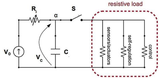
Figure 2: Model of ODC-MFC energy generation. The lumped parameters  $V_0$ ,  $R_i$  and  $C$  schematically represent our platform independent model. A dashed rectangle represents the robot as a resistive load.
