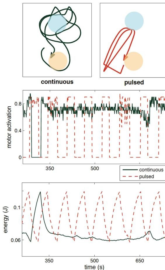
Figure 4: *Top panels*: examples of continuous (green) and pulsed (red) robot trajectories. In each panel, on entering the higher/lower circle the robot receives hydration/fresh substrate. *Lower panels*: motor activation (top) and energy level (bottom) for continuous (continuous green plot) and pulsed (dotted red plot) behavior. Adapted from (Montebelli et al. 2010).
