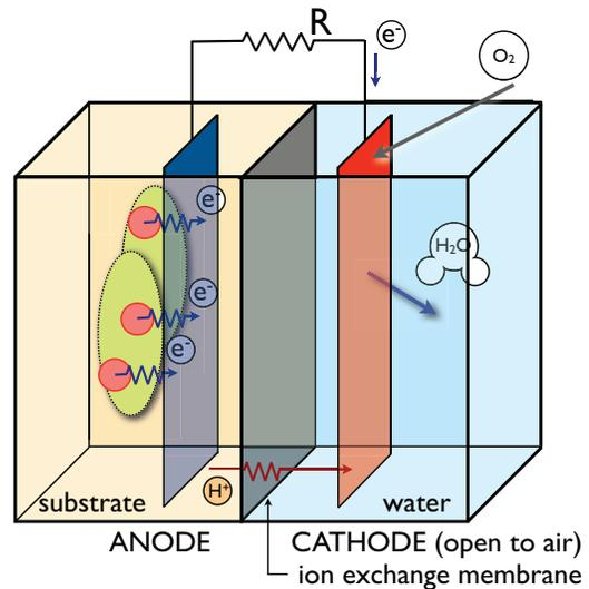
Figure 1: Schematic of an oxygen-diffusion cathode MFC.
