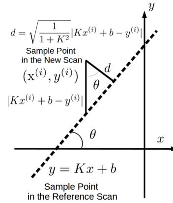
Figure 7: Perpendicular Distance for the Point away from the Line
