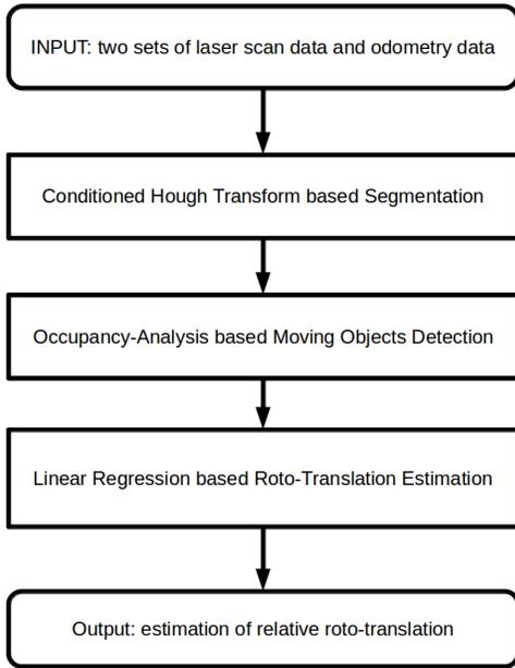
Figure 2: Overview of the Phases in Scan-matching Algorithm
