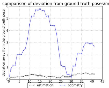
Figure 11: The Comparison of the Deviations from Ground Truth for Estimated Results and Odometry
