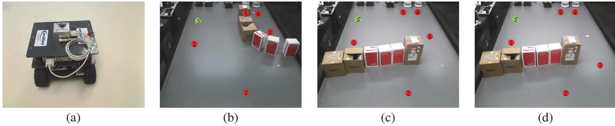
Figure 3: (a) Photograph of Corobot robot used for experiments, (b)-(d) Three environments, each with the same five waypoints (tasks) but different distributions of obstacles used in our experiments. The green circle marked 'S' is the robot's start location and the red, numbered circles show the different waypoints.
