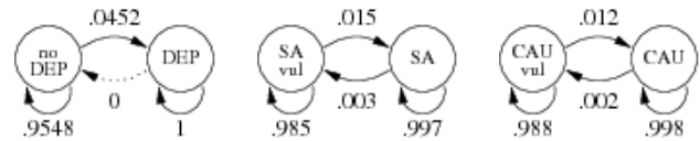
Figure 1: The three independent Markov chains used to model the update mechanism in our example network.
