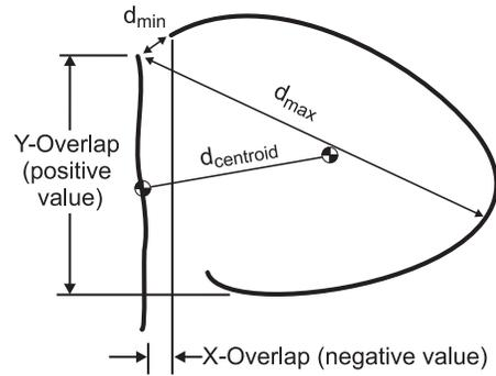
Figure 2: Features used by clustering classifier.
