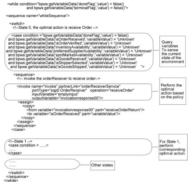
Figure 4: A snippet from the resulting BPEL4WS flow deployed in IBM BPWS4J Workflow Engine. The flow
