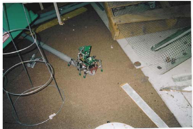
Figure 6. The nylon roller mount on one of the BoeBots (the nylon roller is not installed in the crawler configuration) gets stuck on the end of a pipe in the red area of the USR arena.
