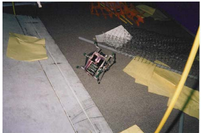
Figure 7. One of the Blue Swarm 2.5 BoeBots has flipped over while trying to climb up the ramp in the orange area.
