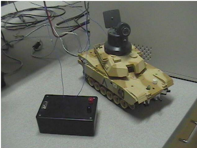
Figure 3. The Blue Swarm Sentinel and its base station RF module.
