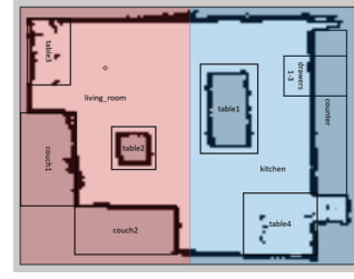
Figure 6: Metric map with an overlay of the spatial volumes associated with nodes in the topological map.
