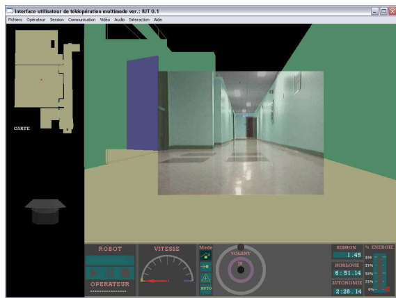
Figure 4: User interface with augmented video display.
