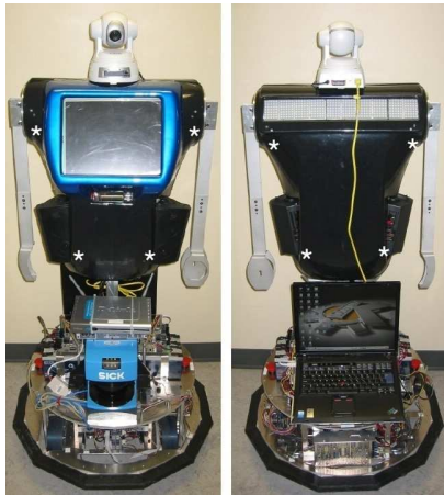
Figure 3: Spartacus (front view, back view), with the microphones located near the *.
