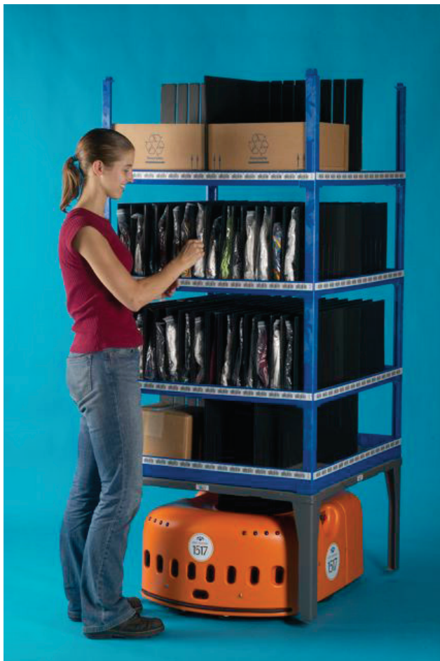
Figure 2: A Kiva drive unit and storage pod.
