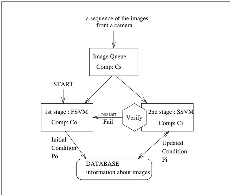
Figure 7. Two-Stage Visual Tracking Method.
