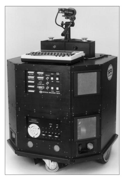
The distributed architecture and loosely coupled control structure enable FLAKEY to simultaneously interpret sensory data, react to the local environment, and form long-range plan. CARMEL was distinguished by its graceful motion around obstacles in open terrain and was pleasant to watch produced and integrated modules for complex behaviors, tasks, and navigation.
