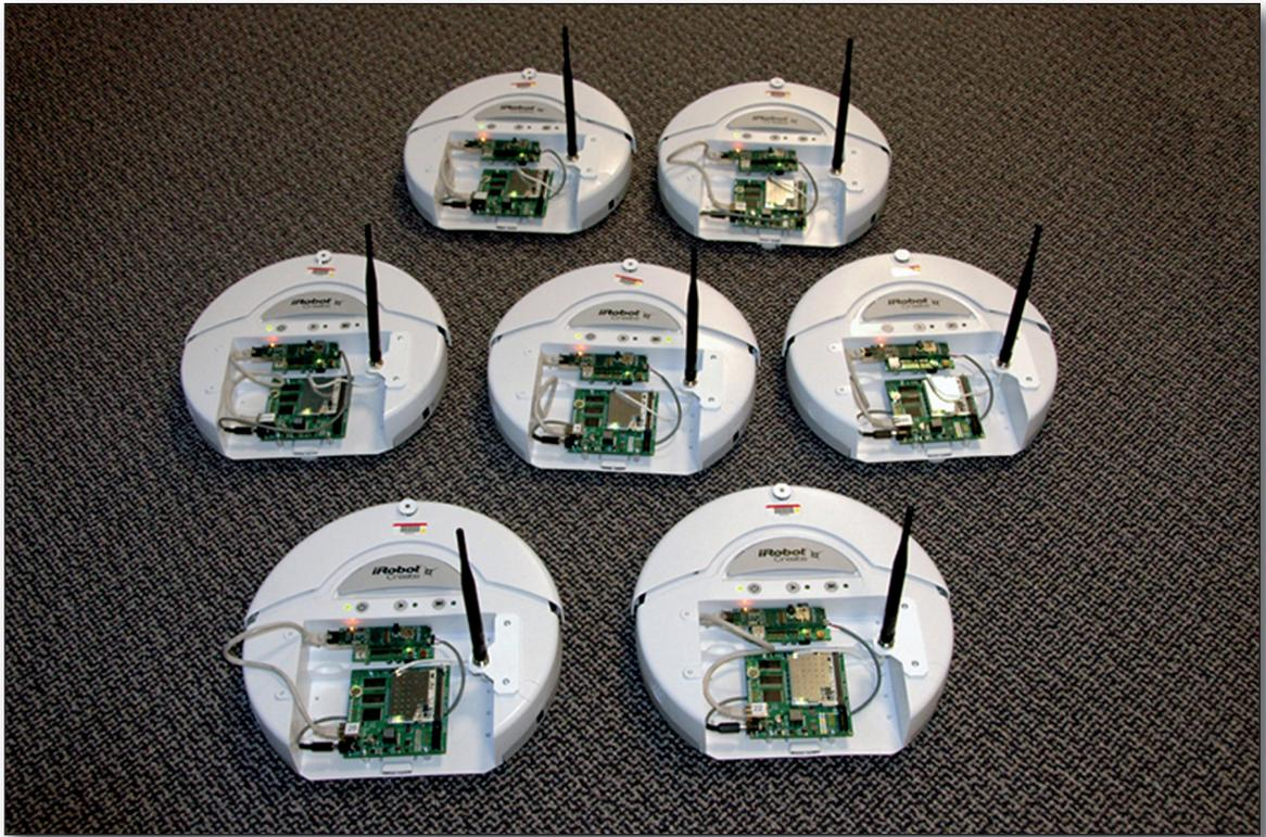
Figure 1. Mobile WLAN Access Points.
