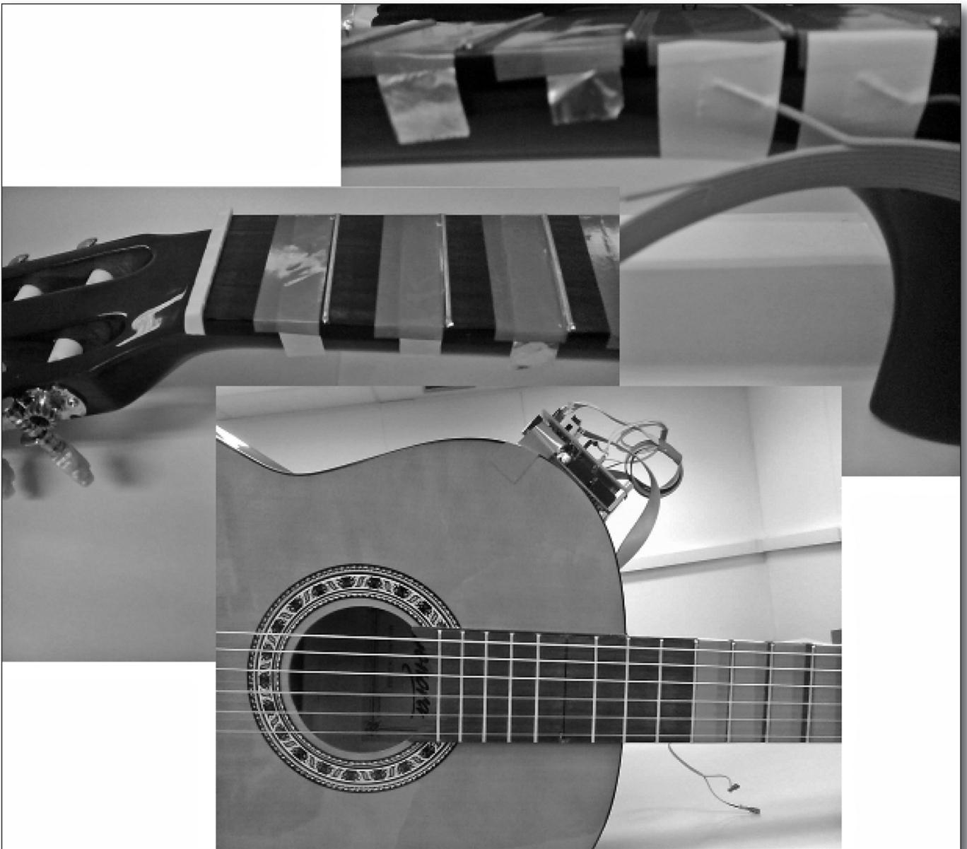
*Figure 4. Nonintrusive Capacitive Sensors Mounted on the First 10 Frets of a Nylon Strings Guitar.*
