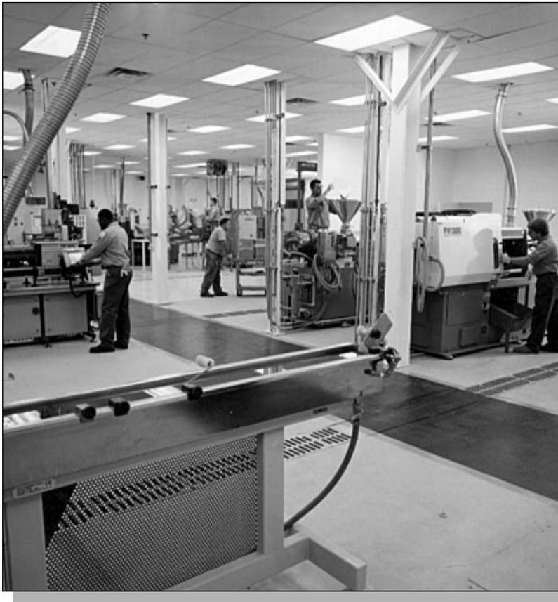
Figure 5. Color Chip Test Molding Machines.
