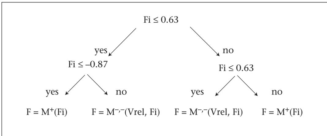
Figure 4. A Qualitative Controller Induced from the Trace of Figure 3.
