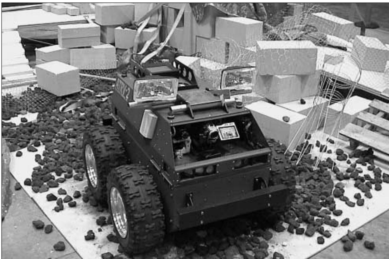
*Figure 5. ATRV Robot in Difficult Section of the Urban-Search-and-Rescue Arena (courtesy of William Adams).*
