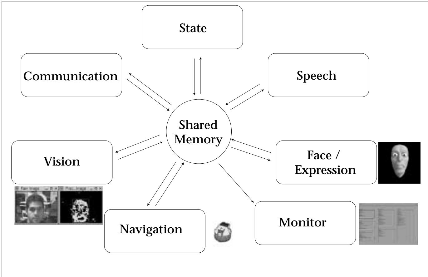
*Figure 2. Logical Diagram of the REAPER Architecture.*
