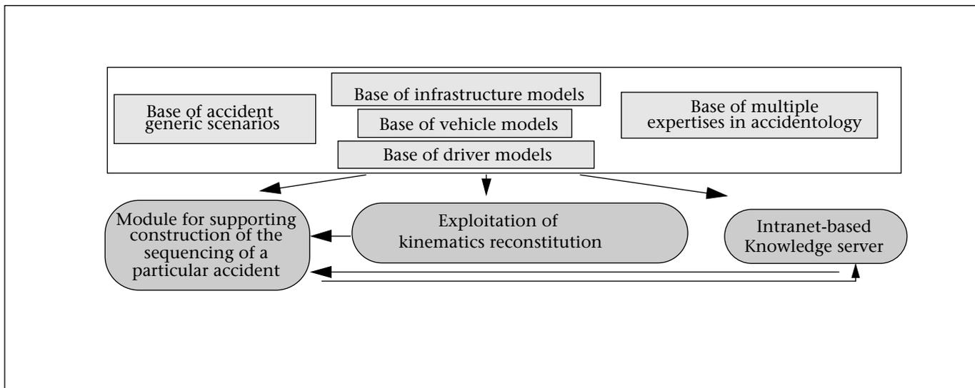
Figure 16. Architecture of the System for Support to Road Accident Analysis.
