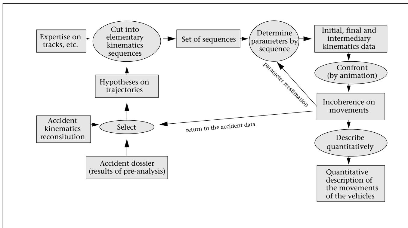
Figure 13. Model of Kinematics Reconstitution for a Vehicle Engineer
