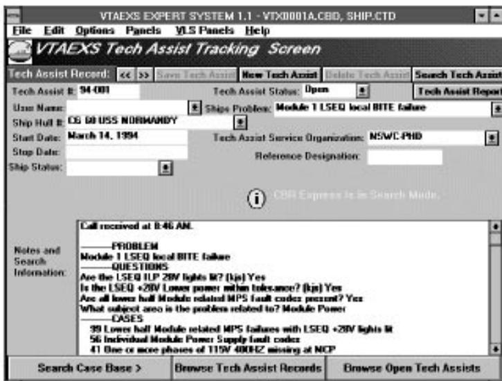
Figure 3. VTAEXS Tech-Assist Tracking Screen.
