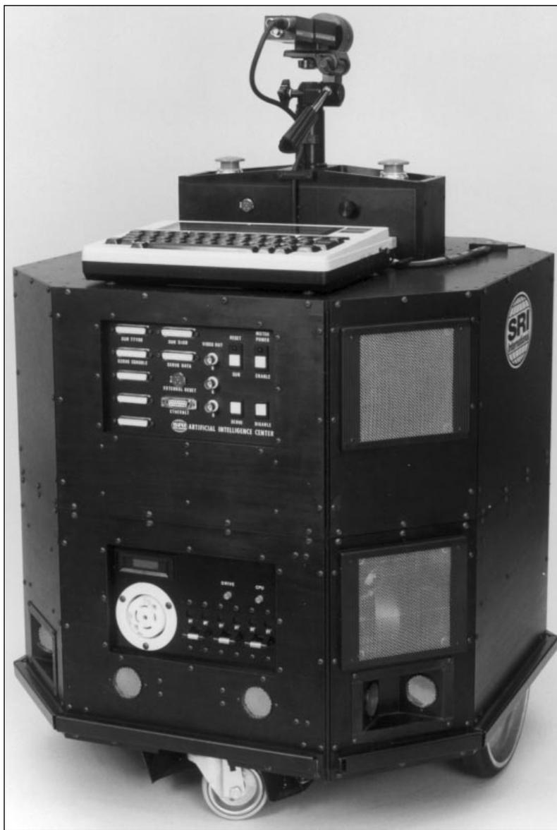
*The distributed architecture and loosely coupled control structure enable FLAKEY to simultaneously interpret sensory data, react to the local environment, and form long-range plans.*
