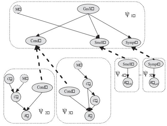
Figure 2: Modular model of the gas monitoring process in Figure 1. Dashed arrows denote the message flow between the collaborating modules.
