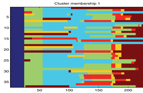
Figure 3: A membership plot. There are 5 clusters in this plot. Time in hours is on the x-axis, host index on the y-axis. Color indicates the cluster to which the host belongs at that time. The solid-colored portion on the left corresponds to the one-day burn-in period, where clustering is not performed. At the end of the run, most hosts lie in the reddish cluster because they have been infected.
